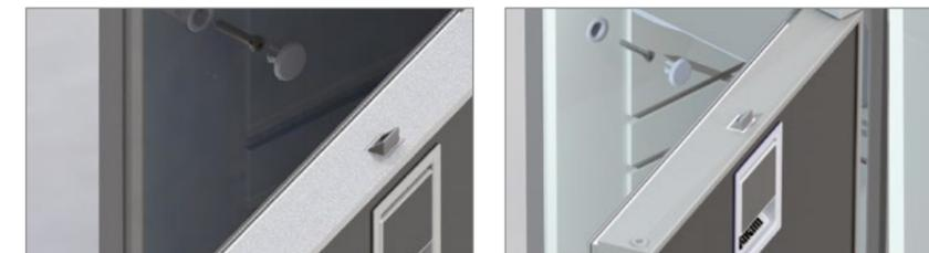
The installation system allows an easy fixing of the cabinet directly from the interior of the fridge. An external flange is not necessary for the installation. An innovative internal bushing structure prevents the crushing of the insulated side wall.
