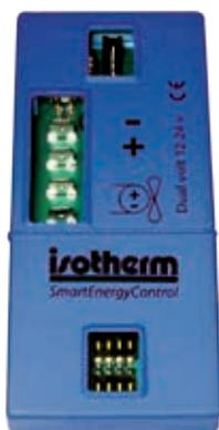
The Smart Energy Control (SEC) is a sophisticated processor-based control device, that achieves significant power consumption by continuously scanning a set of key environmental factors, to operate the compressors at their best performance/battery drain ratio. Via the storage function in food and drinks can achieve up to 50% savings Vs. conventional control systems, representing the best answers for users hunting for the lowest power consumption.
